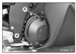
OConnect the KDS (Kawasaki Diagnostic System) connector cover to the original position when the cover is disconnected.
