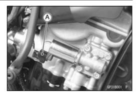
• Set the hand tester [A] to  $\times 1 \Omega$  range and connect the tester leads to the terminals in the oil control solenoid valve lead connector [B].
