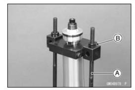
• Insert the compression shaft [A] and install the nut [B]. OSet the other side compression shaft same process.
