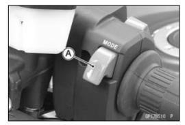
• By pushing the lower button [A] each time, check that the display [B] changes as follows.
